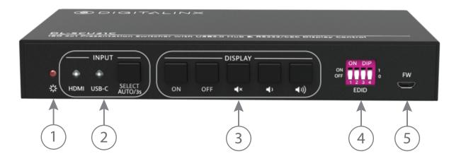
1. POWER LED - Illuminates solid RED when power is properly applied
